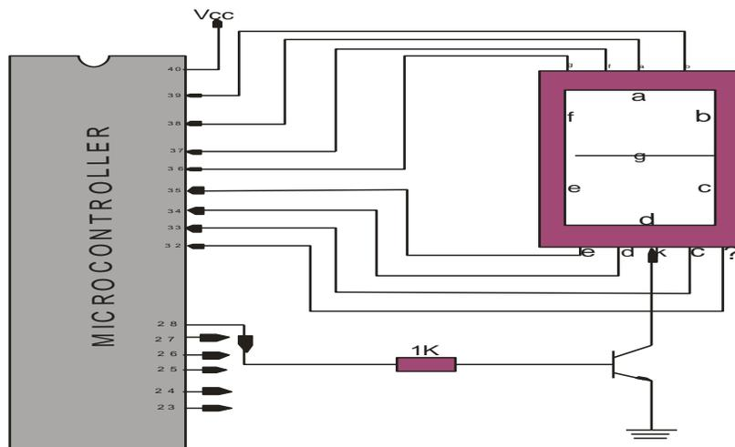
Fig 7: The diagram of 7-segment display interfacing a microcontroller
