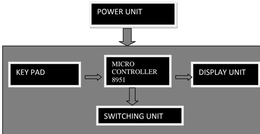
Fig.10: Block Diagram Micro Controller Power regulated unit
