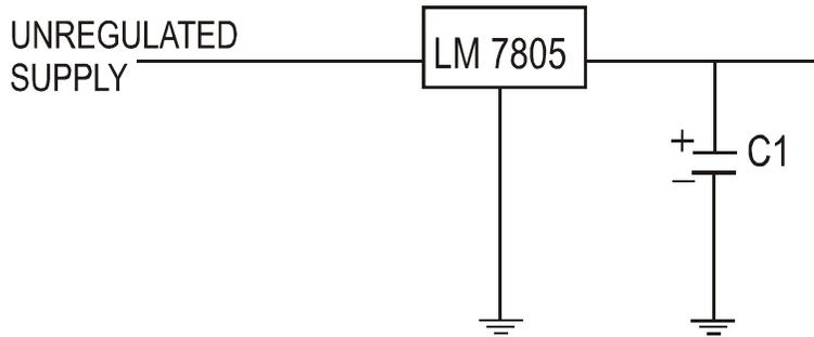
Fig 6: Constant 05 volts circuit using LM7805
