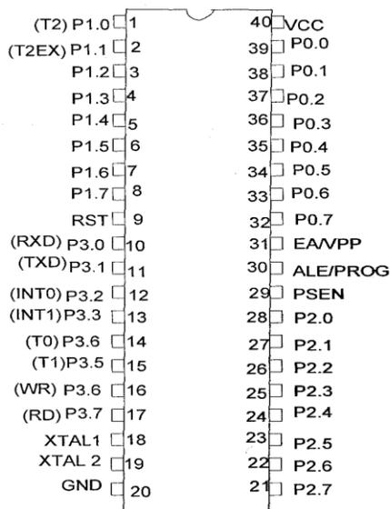
Fig 1: The AT89C52 chip
