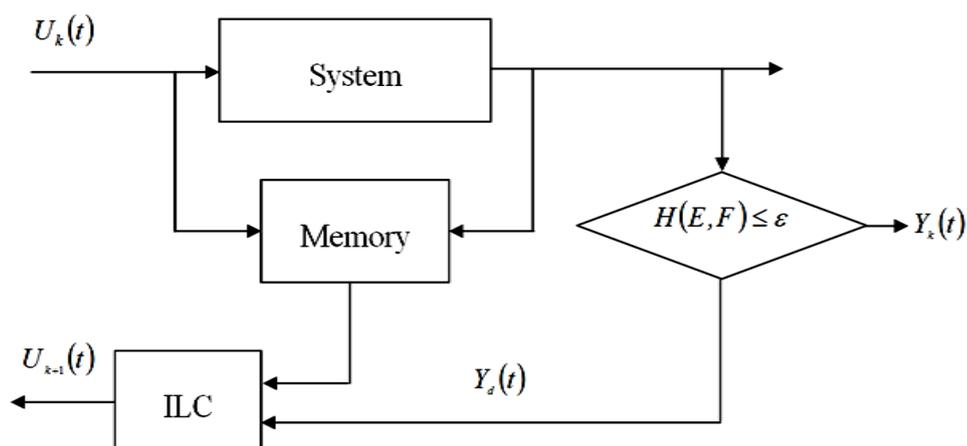
Fig. 1. The basic scheme of iterative learning control with  $Y_d(t)$  being the trajectory,  $U_k(t)$  and  $Y_k(t)$  the input and output signals.
